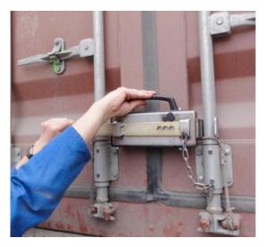
d. Move the sliding bar to its closed "position". Then place the magnetic pin in the locking hole that leaves the sliding bar with the least movement possibility.
