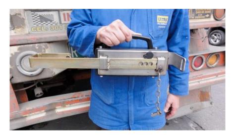
c. Install the Lock in the right hand side central container bar as shown in the picture, and then move it forward in between both container bars.
